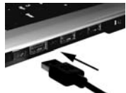
3.2: Connect the cable's other end to a laptop or other USB 2.0 charging port
